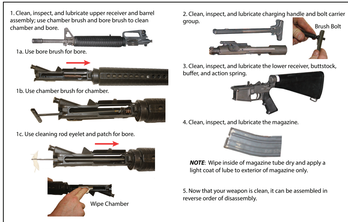
Figure 7.11 M16A2/M4 Cleaning Procedures
